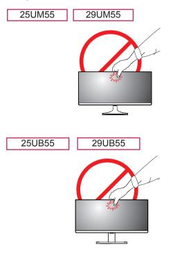
If you use the monitor panel without the stand base, its joystick button may cause the monitor to become unstable and fall, resulting in damage to the monitor or human injury. In addition, this may cause the joystick button to malfunction.
